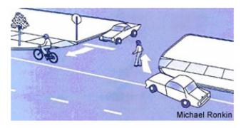
Radius type driveways allow higher motor vehicle speeds. Driveways should NOT be designed like this.
