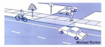
Wing-type driveways provide the best pedestrian crossing as long as the driveway apron does not extend into the sidewalk area.
